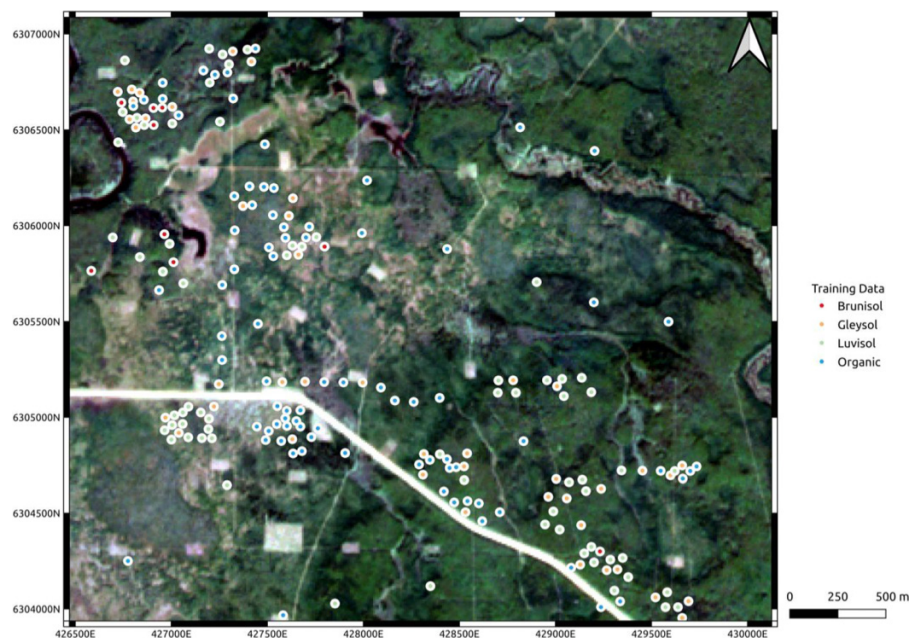
Fig. 2. True color red–green–blue 2015–2020 median reflectance (Sentinel-2 bands 2, 3, and 4) for an example area within the larger study area (European Space Agency 2021). The points correspond to soil sample data (training and testing point data) that were collected within this area. Coordinates are in UTM Zone 12N NAD 83. [Colour online.]
