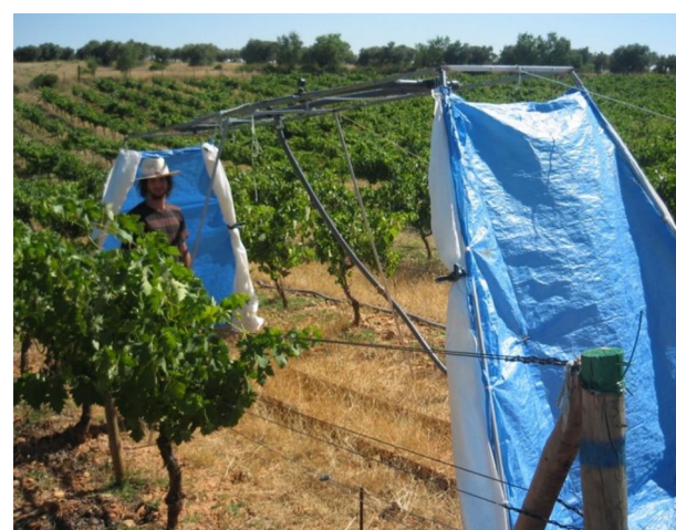
Figure 2. Rainfall simulator. Two full cone nozzles placed in an operating height of 2 m above ground. The windbreaks are partially placed around the simulator in the picture. During the experiment, the windbreaks were unfolded completely for preserving rainfall distribution.
