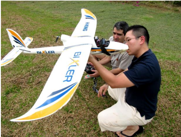
Fig. 1. The prototype of the Conservation Drone used in test missions in Sumatra, Indonesia.
