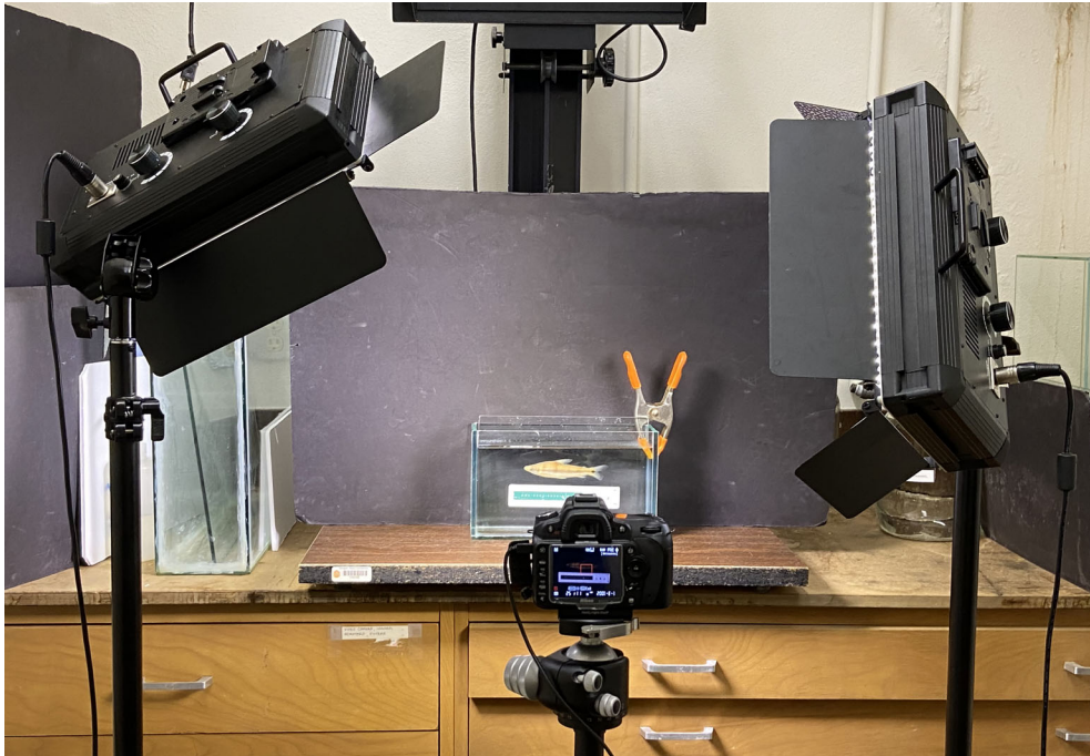
Fig. 3. The photography room at the Oregon State Ichthyology Collection, including photo tanks, LED arrays, camera, and tripod. (Credit: B. Sidlauskas).
