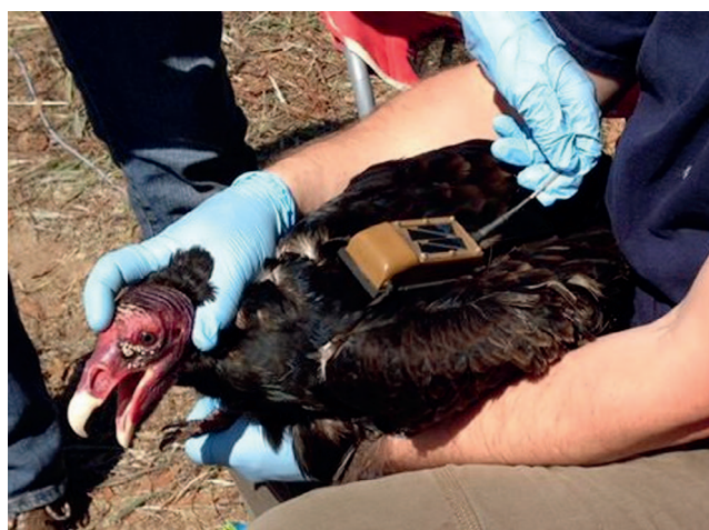
APPENDIX FIGURE 8. Example of a solar-powered GPS-GSM transmitter (Microwave Telemetry, Columbia, Maryland, USA) attached to a Turkey Vulture.
