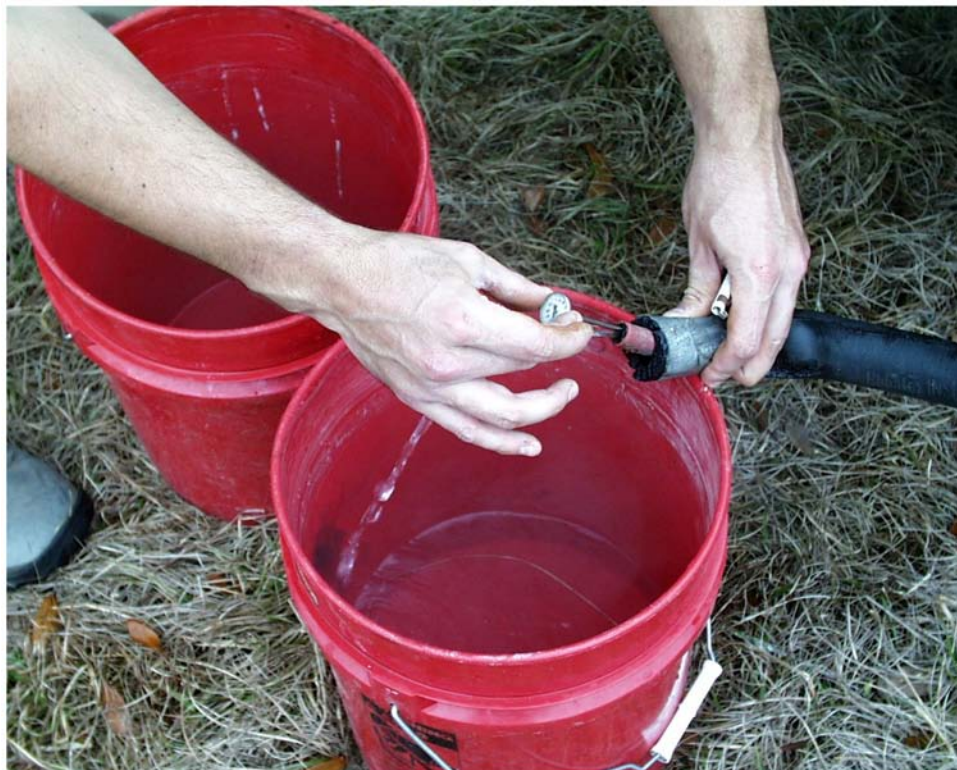
Figure 8. Measuring the temperature at the hot-water outlet. Knocking down ash and keeping the charcoal topped up assures that the effluent water temperature is always between 60° and 85° C.
