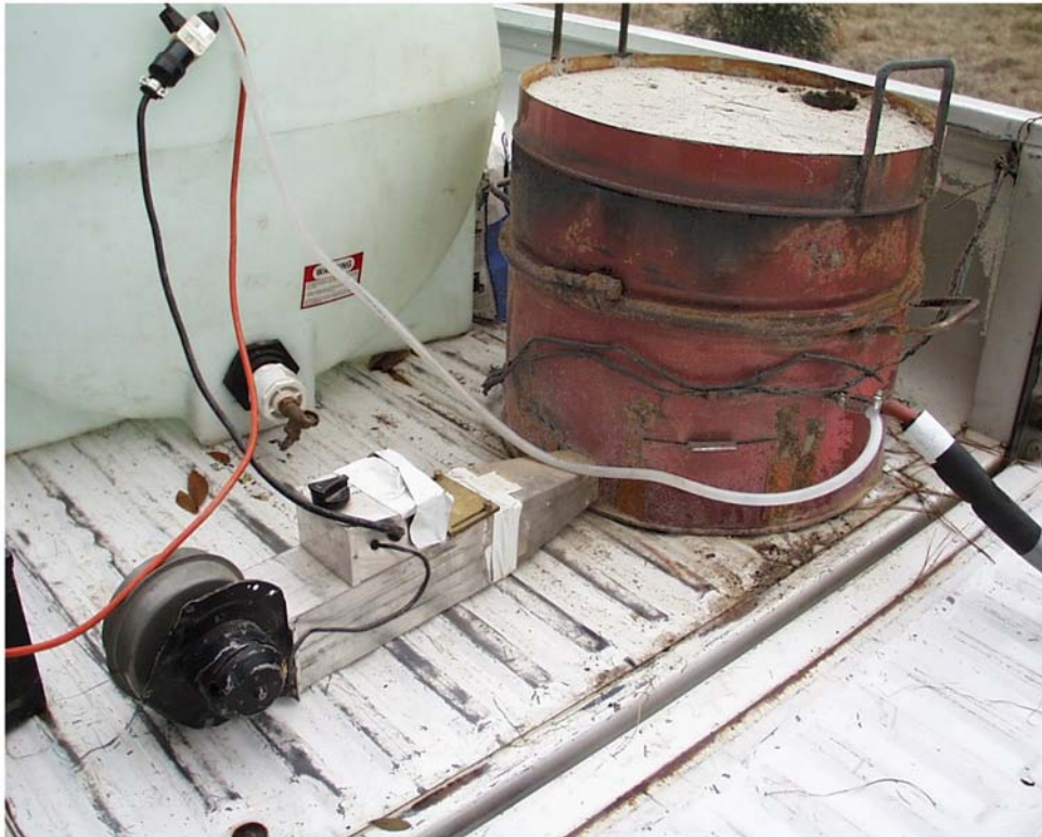
Figure 5. Modified automobile heater fan, powered by a 12-v marine battery. The tapered outlet increases the air velocity entering the bottom of the kiln.
