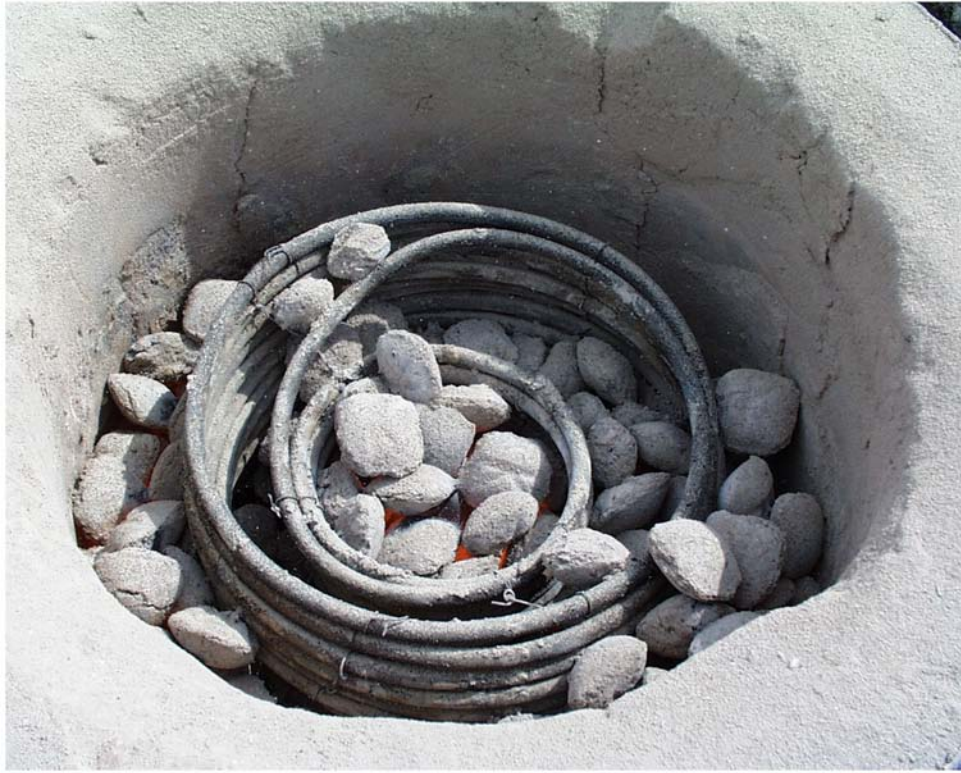
Figure 4. The coil in operation in the kiln, lid removed. Note that charcoal contacts both the inner and outer sides of both coils.
