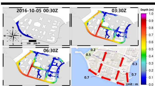
Figure 5. Simulated wave overtopping and inundation spreading pattern with the maximum depth (m) and the field survey results (lower right image).
