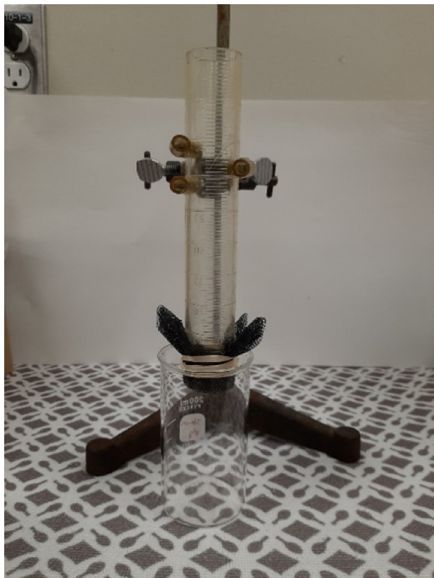
Fig. 3. Water retention measurement apparatus.
