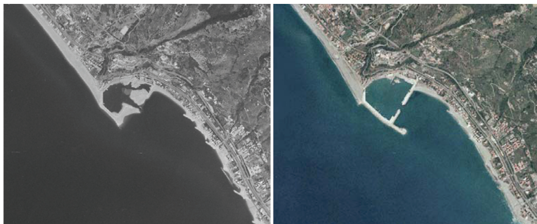
Figure 3. Aerial view of the Cetraro Port in 1988 before the dredging, and in 2000 after the dredging.
