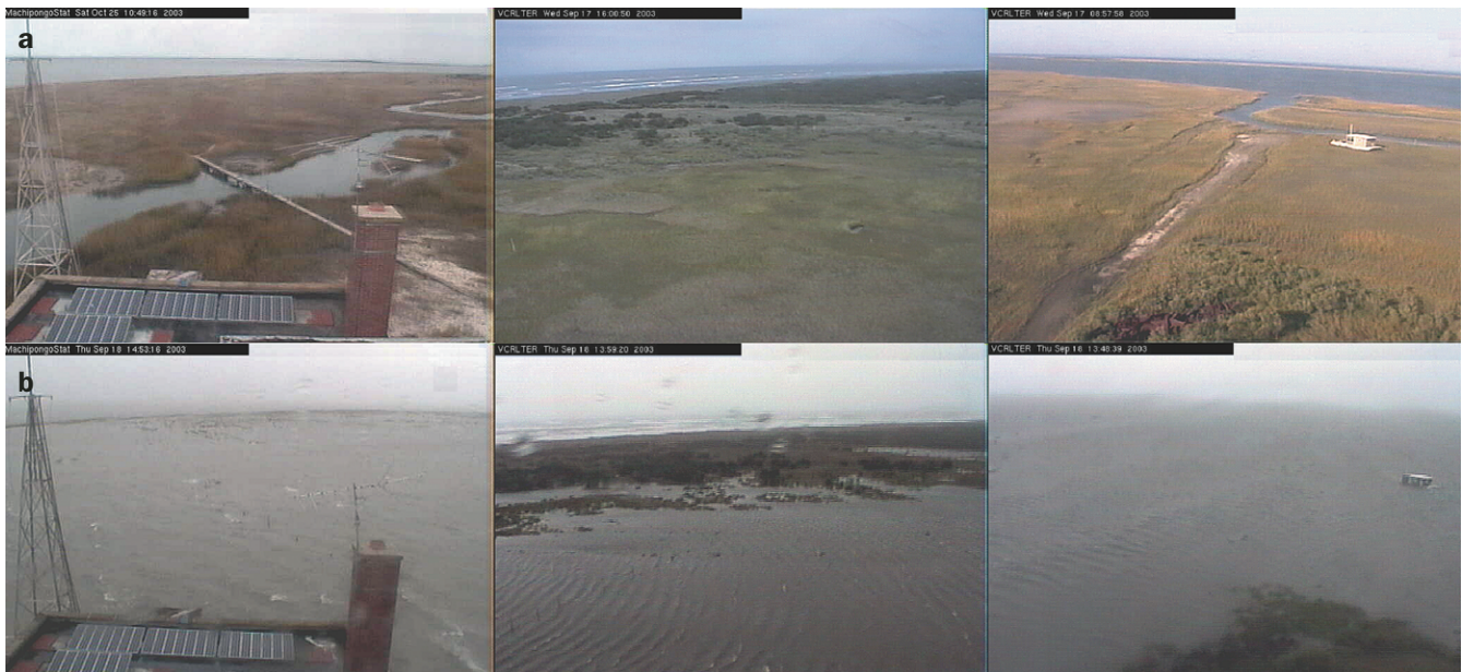
Figure 5. Images from wireless cameras (a) before and (b) during Hurricane Isabel (18 September 2003). Researchers increased the image sampling rate during the storm from an Internet café in Seattle. The network continued to provide image and meteorological data throughout the storm until a power failure occurred in the mainland laboratory. Photographs: John Porter.
