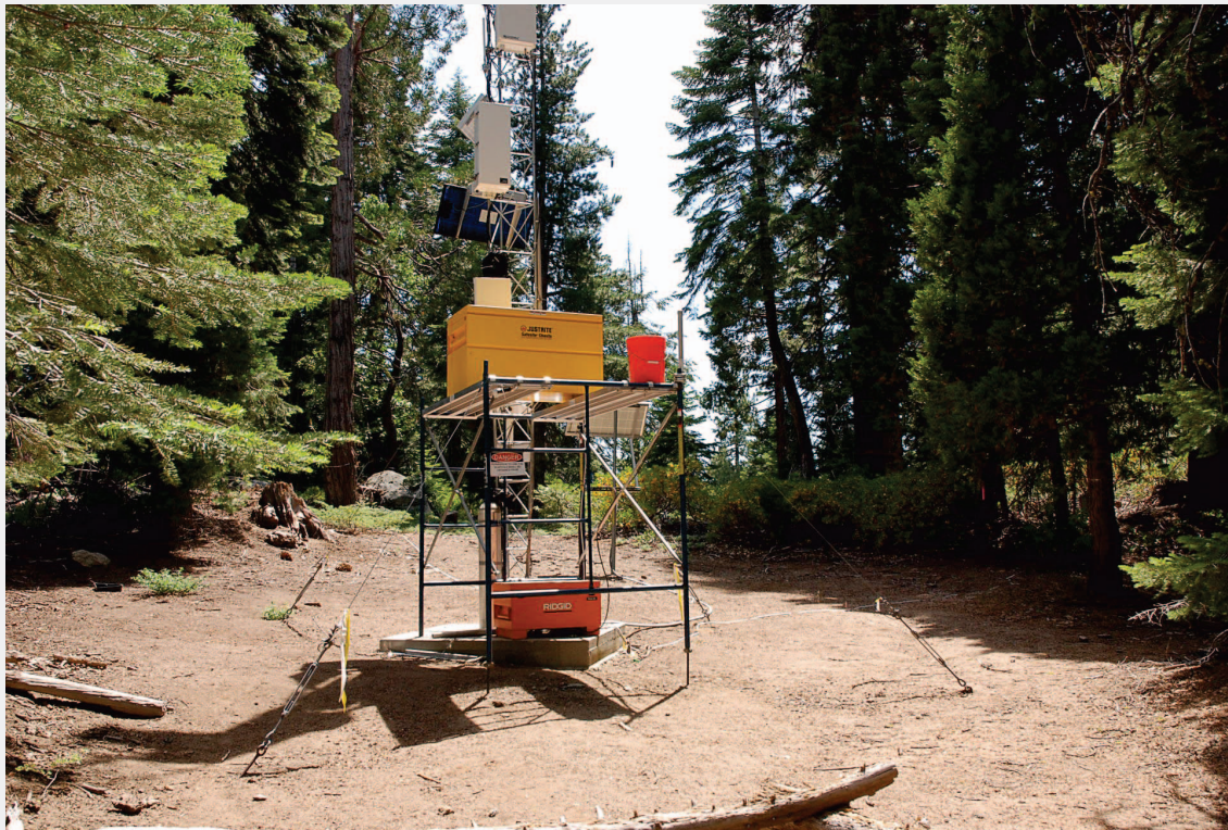
FIGURE 1 One of four flux towers installed at different altitudes between 405 and 2700 m by the Southern Sierra Critical Zone Observatory, California, USA. Instruments collect information about climate and fluxes of carbon dioxide and water vapor with the objective of gaining new knowledge on how water, soils, and climate interact. (Photo by Claudia Drexler)
