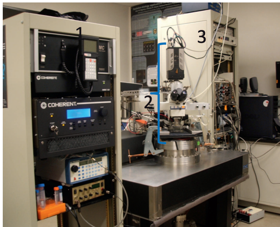
FIG. 5. The electrostatically focused single-particle microbeam facility in the new microbeam laboratory (Microbeam II): 1. The control electronics for the multiphoton laser; 2. the microbeam stage, microscope and camera; 3. the electronics rack containing instrumentation for the microbeam.
