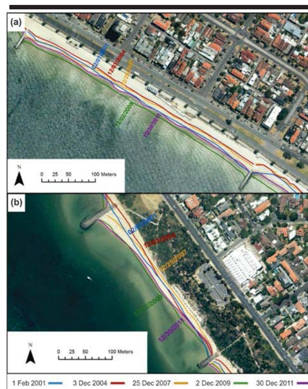
Figure 4. (a) Shoreline change at Middle Park between 2001 and 2011, showing shoreline accretion due to renourishment in 2009 (green line), followed by subsequent erosion (pink line). (b) Shoreline orientation at Sandringham as influenced by the construction of the northern groyne in 2006; the blue and red lines show the pre-groyne shoreline orientation. This area was also renourished in 2009.
