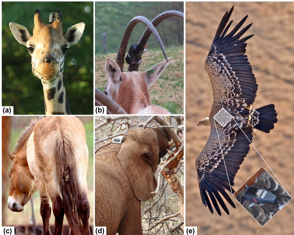
Figure 5. Trials of the solar-powered device showing a range of attachment types across taxa including (a) giraffe – ossicone, (b) scimitar horned oryx – horn (© John McEvoy/SCBI), (c) Przewalski's stallion – tail hair (© John McEvoy/SCBI), (d) elephant calf – collar (© David Daballen) and (e) Rüppell's vulture – 'backpack' (© Laila Bahaa-el-din; inset: Henrik Rasmussen).
