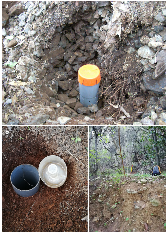
Fig. 1: Details of MSS traps. a. Filling stones into the hollow around a PVP pipe sealed by a silicone cap installed in the MSS; b. Detail of the collecting tray filled with propylene glycol, with a bait container placed in the centre. A nylon cord is tied to the bait container to descend and lift the tray through the PVC pipe; c. Landscape/vegetation at Brezal del Palmital. Photos: H. López
