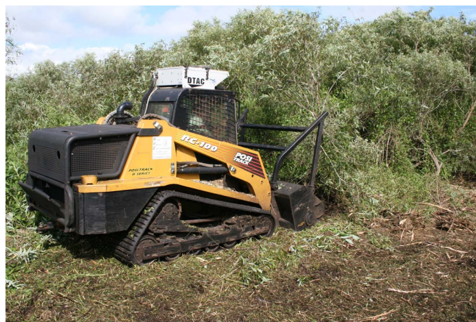
Figure 8. —Rubber track skid steer with a gyro trac mulching head mulching willow at Corkscrew Swamp Sanctuary.
