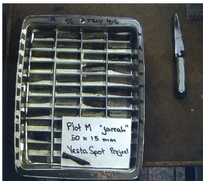
Plate 1 Jarrah samples, each 50 mm long and 15 mm wide, stored in a tray prior to testing in the CSIRO Bushfire Behaviour and Management Group vertical wind tunnel.
