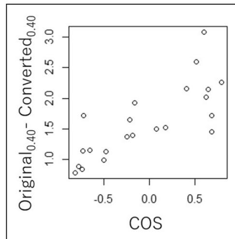
**Figure 7.** Plot of the difference between the original<sub>0.40</sub> and converted<sub>0.40</sub> values against the cosine of the angle formed by the solar azimuth and slope direction.
