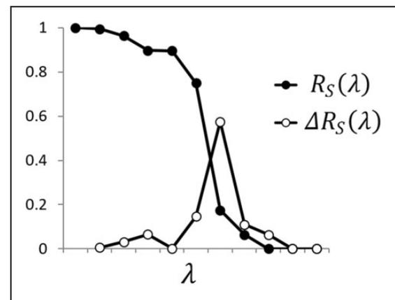
**Figure 5.** An example of granulometric analysis on the image from Figure 4. Plot of the sum of the gray values of the opened image divided by the sum of the gray values of the original image ( $R_S(\lambda)$ ) and the difference ( $\Delta R_S(\lambda)$ ) with regard to the radius of the structuring element ( $\lambda$ ).
