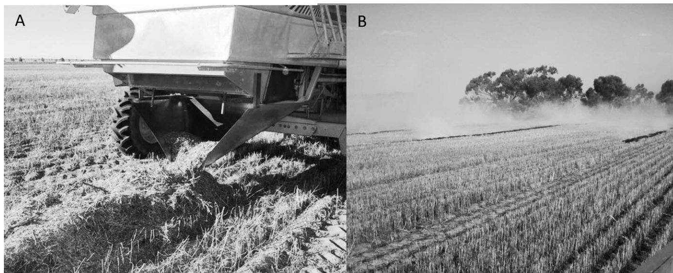
Figure 2 a) Chaff chute mounted on the rear of a harvester to form narrow windrows during harvest. b) Burning narrow windrows in wheat stubble in autumn (March to April)
