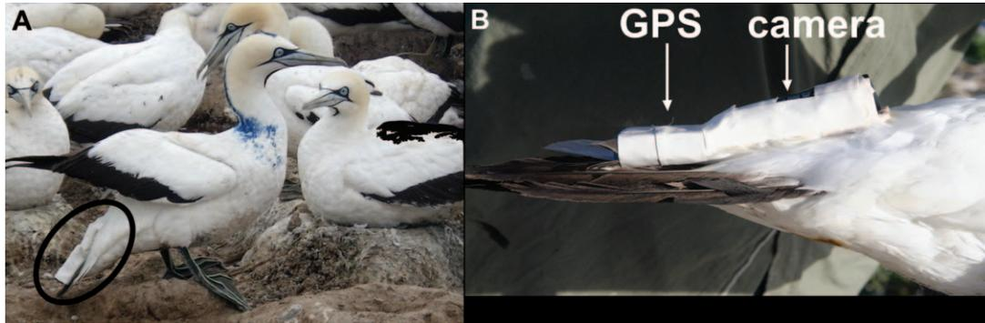
**FIGURE 2.** Photographs of the devices attached to Cape Gannets. (A) The devices are located on the lower-back and tail feathers of the bird. (B) A closer view, showing both the GPS device and the micro video camera.
