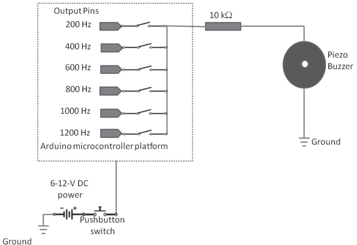
Fig. 1. Diagram of *D. citri* mimic-signal broadcast device, including the output pins on the Arduino microcontroller platform and the manual switches setting the output to the piezo buzzer. During bioassays, the main power switch was controlled remotely (Pushbutton) from outside the anechoic chamber.
