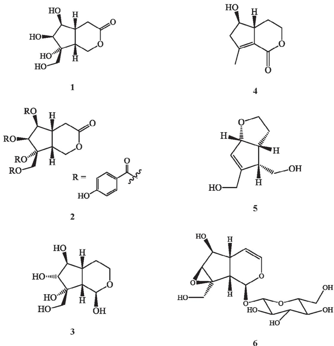
Fig. 1. Iridoids isolated from *Crescentia alata* fruits.
