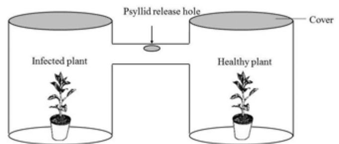
**Fig. 1.** Sketch of H-shaped device for determining the choices of *Diaphorina citri* adults for HLB-infected versus healthy citrus plants either in darkness or in normal illumination. The device was made of an opaque plastic, and the cylinders were covered either with 2 black paperboards or with 2 transparent plastic boards.
