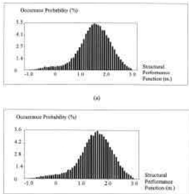
Figure 3. Frequency simulation of the structural performance function at the limit state for the duration of 100 years. (a) Case I: Tsunami risk not considered (b) Case II: The effect of tsunami risk.
