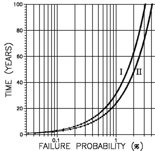
Figure 4. Failure probability of the breakwater as a function of time. I: No tsunami II: Tsunami risk included.
