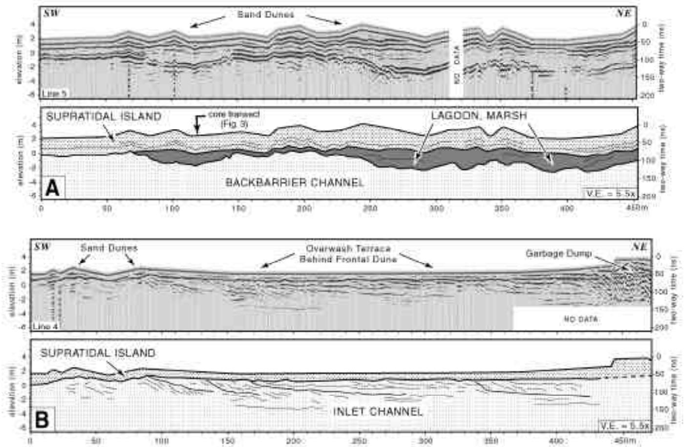
Figure 4. Ground-penetrating radar (GPR) profiles from central Tavira Island. A) Shore-parallel profile across dunes near the center of relict delta complex. B) Shore-parallel profile across flat overwash terrace located just behind frontal dune. See Figure 3 for location of profiles. Frequency is 100 MHz; velocity is 0.1 m/ns.
