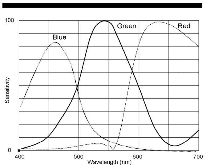
Figure 8. Approximate CCD spectral sensitivities. After Sony (2000)
