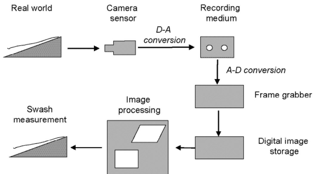
Figure 3. Video imaging and measurement process (after CLARKE *et al.*, 1995)). This schematic illustrates an analogue system. Digital (IEEE1394) systems remove the D-A-analogue recording and frame grabber stages from the post-processing environment.
