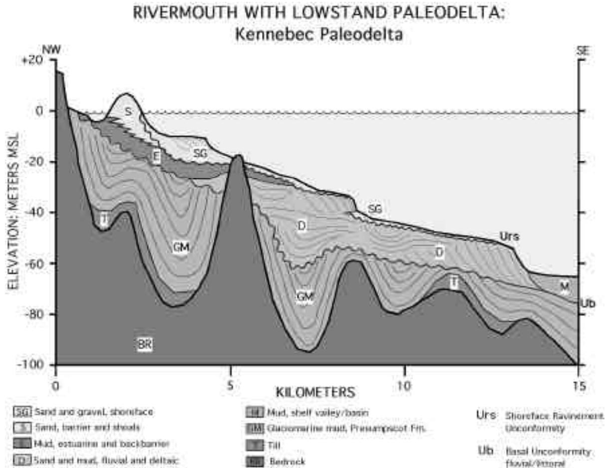
Figure 7. Schematic representation of inner shelf stratigraphy off a large river mouth with a lowstand paleodelta: Kennebec Paleodelta (after BELKNAP *et al.*, 1989, BARNHARDT *et al.*, 1997). Basal unconformity Ub is the lower sequence, separating glacial and glaciomarine units from transgressive marine and coastal facies. D represents lowstand and mid-shelf paleodelta systems. E represents estuarine and backbarrier facies of mid-to-late Holocene barrier and river-mouth systems.
