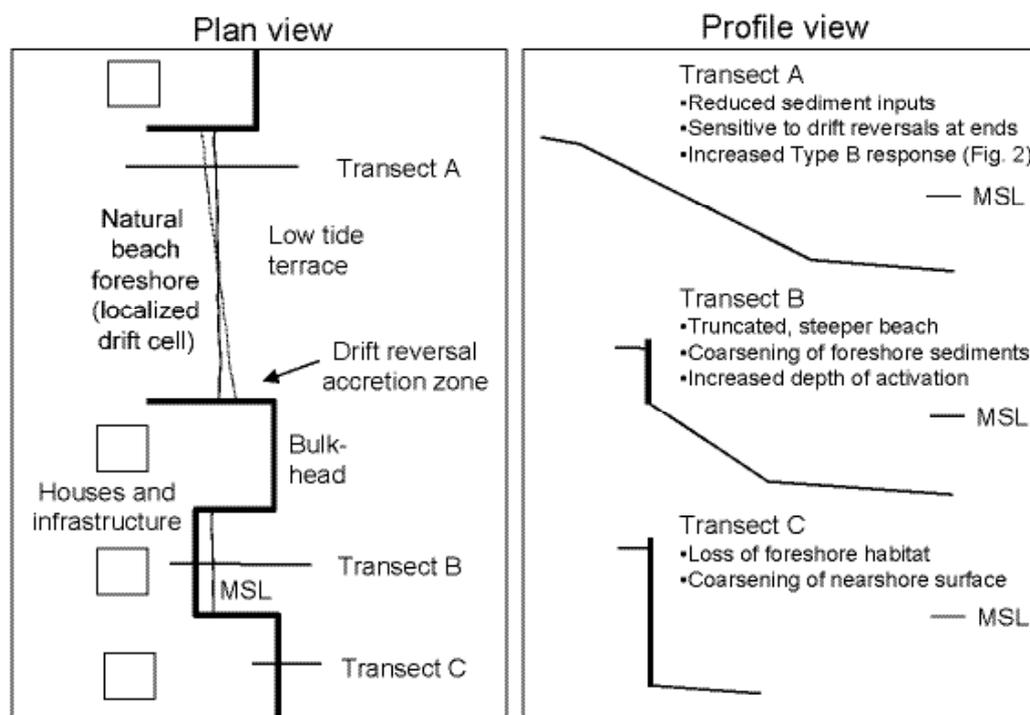
Figure 4. Effect of bulkheads on an estuarine shore.
