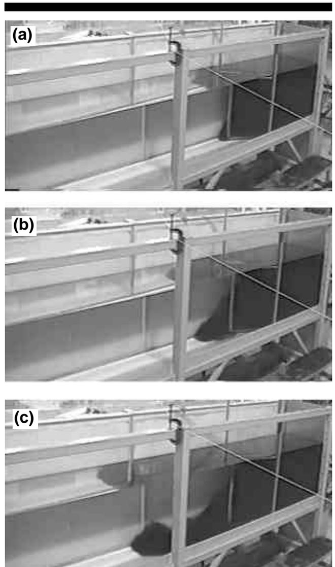
Figure 3. Spreading behaviour of a lock water into the tank for  $V = 0.022 \text{ ms}^{-1}$  and  $UT = 0.11 \text{ ms}^{-1}$  and  $H = 0.5 \text{ m}$ . The images were recorded at times corresponding to (a) 10 sec, (b) 14 sec and (c) 24 sec after the gate opening process commenced. NB. The spreading rate velocities are not presented in this paper.
