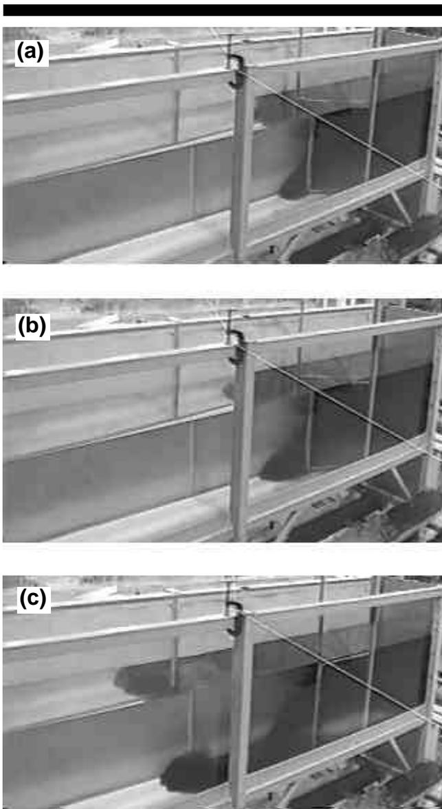
Figure 4. Spreading behaviour of a lock water into the tank for  $V = 0.24\text{ms}^{-1}$  and  $UT = 0.11\text{ms}^{-1}$  and  $H = 0.5\text{m}$ . The images were recorded at times corresponding to (a) 0.1 sec, (b) 3 sec (c) 6 sec and (d) 12 sec after the gate opening process commenced. NB. The spreading rate velocities are not presented in this paper.
