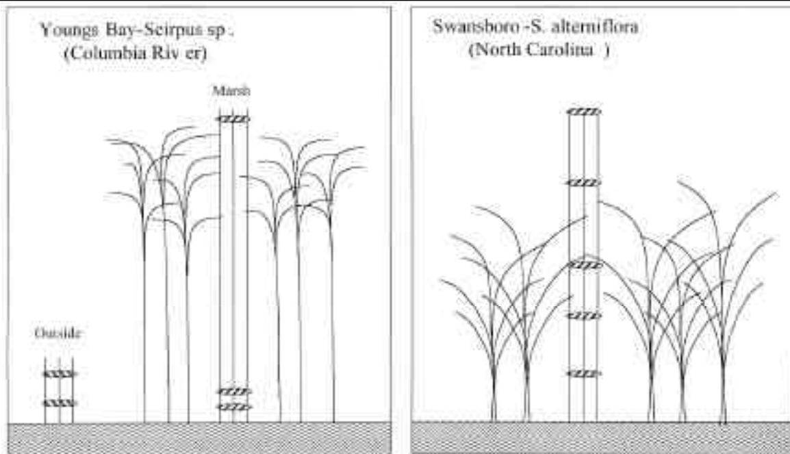
Figure 3. Schematic showing sampling strategy for measuring flow speeds within *Scirpus* sp. (Columbia River, OR) and *S. alterniflora* (Swansboro, NC). Flow data were collected using hot-film anemometry sensors.
