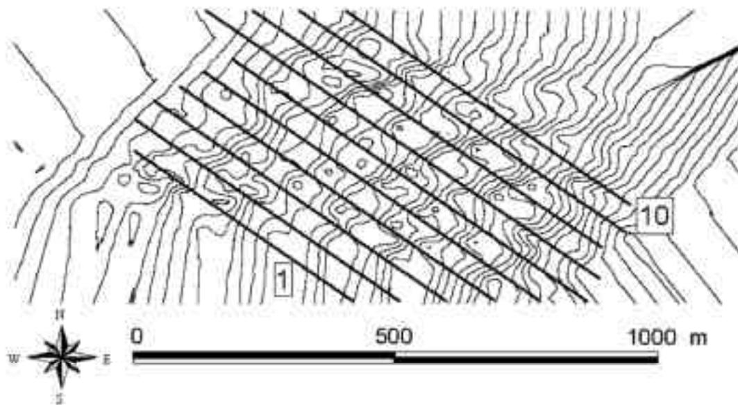
Figure 8. Area no. 1: bathymetry and profile marks.
