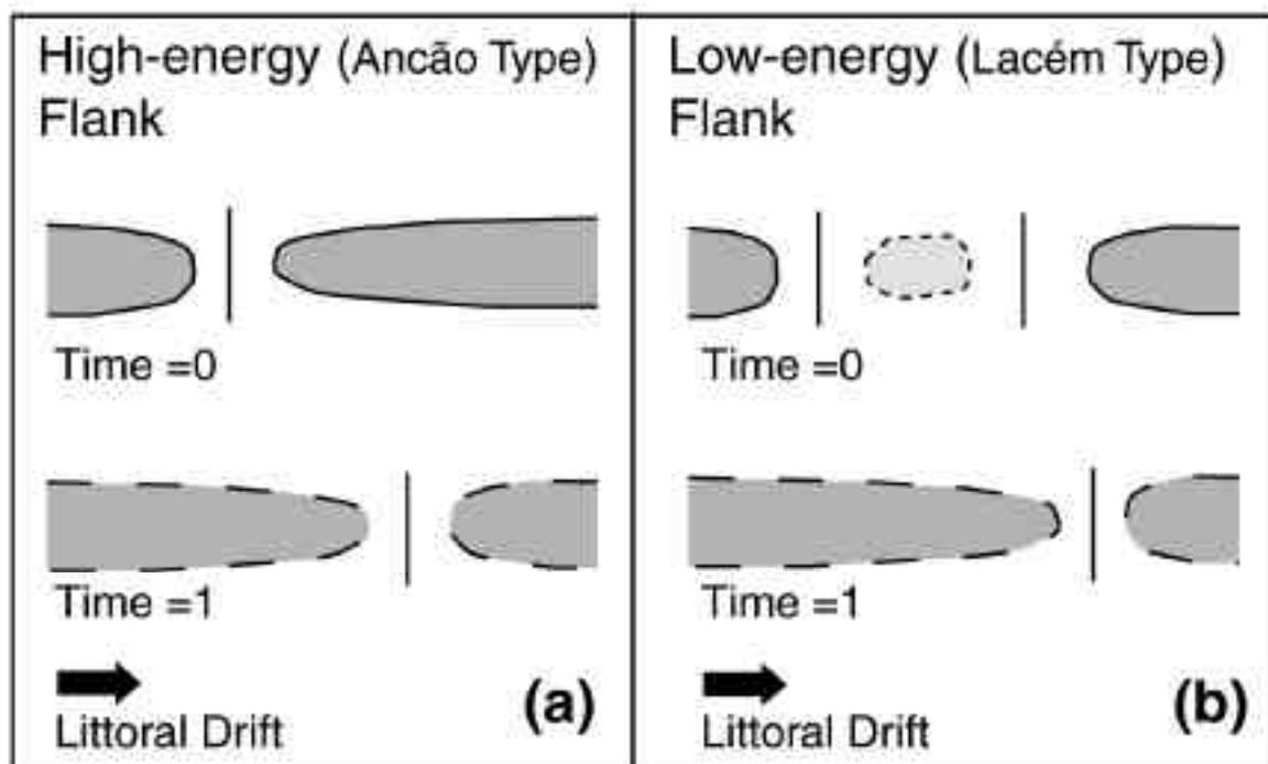
Figure 7. Typical inlet migration patterns determined for the natural inlets at the Ria Formosa barrier island system. (a) Represents the Ancão type of migration, typical for the high-energy flank. (b) Shows the Lacém type of migration, typical for the low-energy flank.
