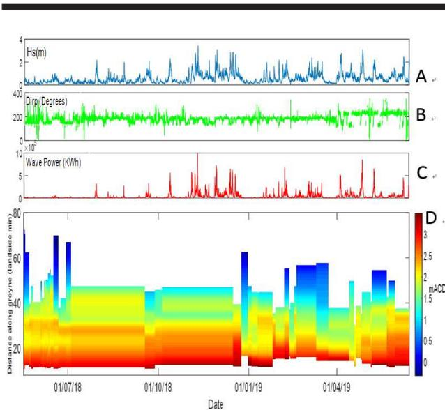
Figure 8. Elevation plot of the 54 profiles. a..Hs, b. wave direction, c. wave power from buoy data obtained by the Boscombe wave buoy up until March 2019 and Poole Bay buoy from April 2019 onwards. Data from Cefas 2019. d. beach profiles (mACD), larger time windows represents period where no other image could be used.
