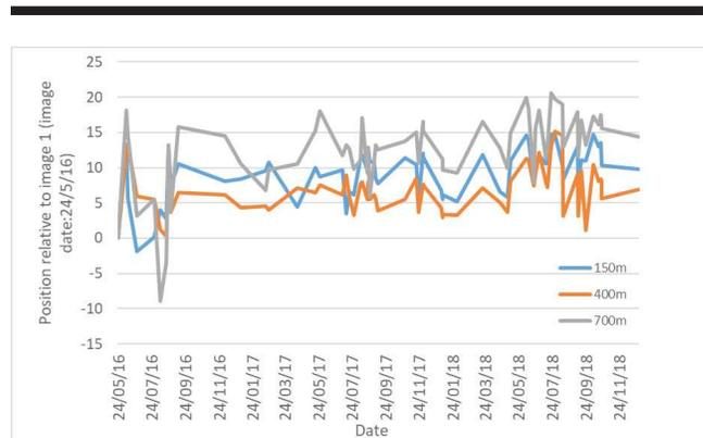
Figure 6. Cumulative pebble toe position at different distances from the camera. Sixty-three (63) images were used. Positive numbers indicate bank retreat and erosion, while negative numbers represent accretion and movement seaward.
