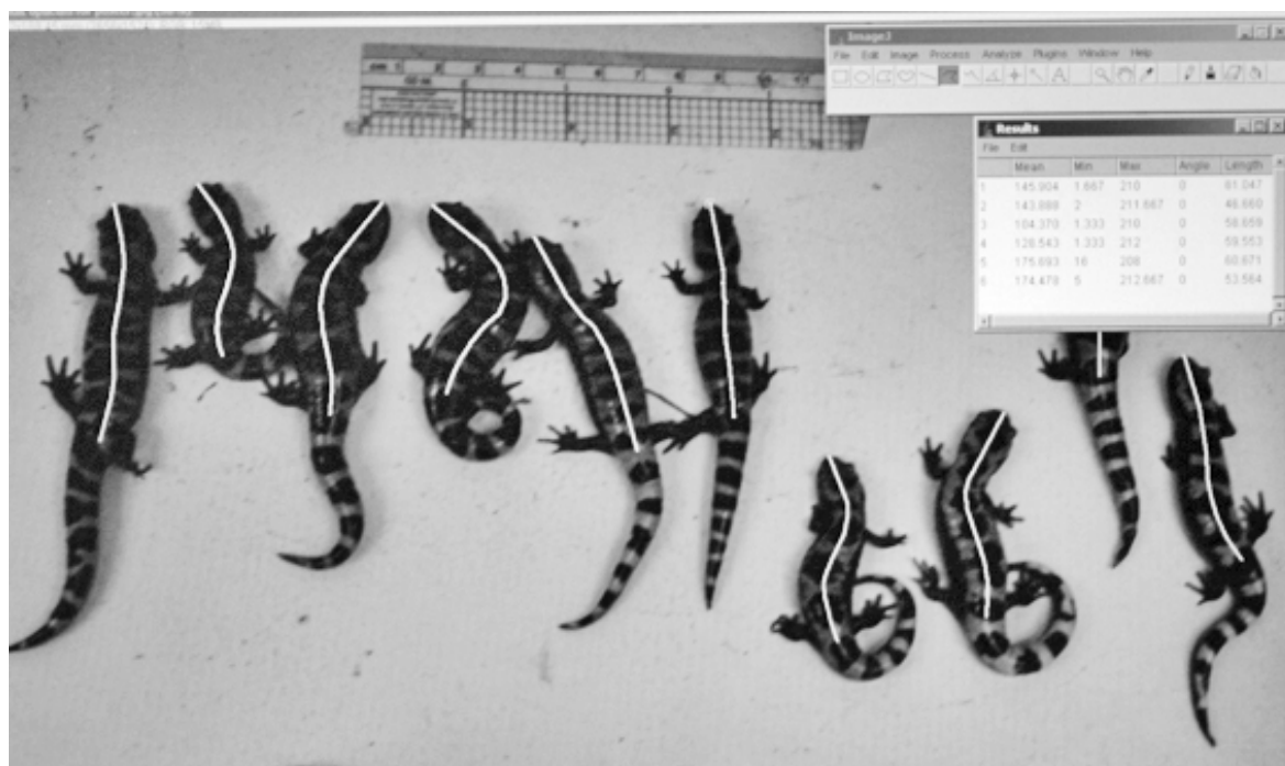
Figure 1. Measurement of adult marbled salamander snout-vent length (SVL) using the 'bent line' function of Image J image analysis software. Plastic rulers are included in each photo for the purposes of calibration, and Image J provides data in tabular form after each measurement (see upper right corner), which can easily be transferred to other formats.
