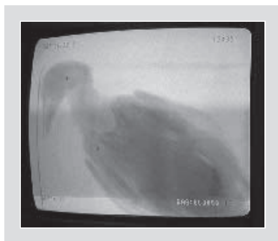
Figure 2. Standard airport security X-ray equipment was used to identify embedded shot. This common eider carries one pellet in the head and one in the breast muscle.
