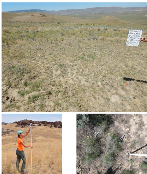
Figure 4. Examples of photos used in monitoring. Top: perspective landscape photograph. Bottom left: capturing aerial photograph from 2 m height. Bottom right: example of the resulting aerial photograph to be digitally analyzed using grid-point intercept.
