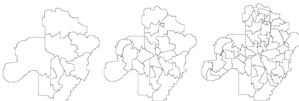
Figure 6. Minnesota SMCW discretized into various sub-basins increments to explore impact of sub-basin scale/HRU density on simulated watershed behavior.
