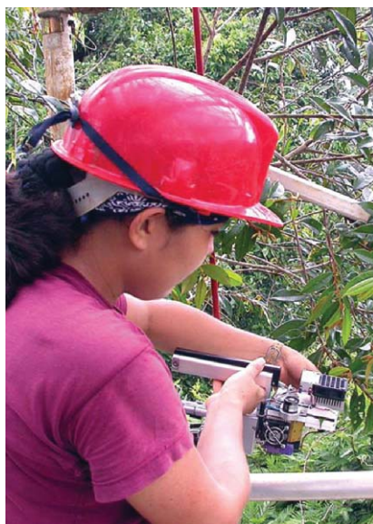
Research assistant Harlyn Ordóñez measures photosynthesis of canopy tree leaves with a portable photosynthesis system at the top of a sampling tower. Frequent measurements of wind speed and direction are combined with measurements of ambient carbon dioxide concentrations to track the exchange of carbon between the forest and the atmosphere. Photograph: Mike G. Ryan.
