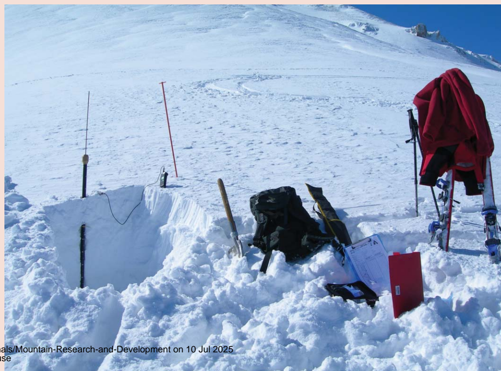
FIGURE 1 Sampling of snow layer for pH and electrical conductivity PROFILE determination in Prati di Tivo, Abruzzo, Italy. (Photo courtesy of Pinuccio D'Aquila)
