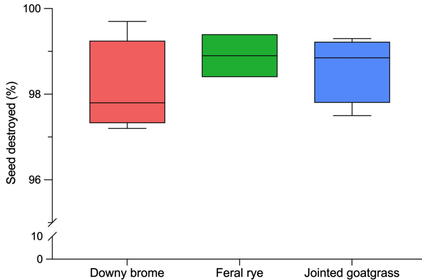
Figure 3. Box plot describing the percentage of seed destroyed by the integrated Harrington Seed Destructor for downy brome, feral rye, and jointed goatgrass, as measured by reduction in seedling emergence compared with untreated controls (see Equation 2).
