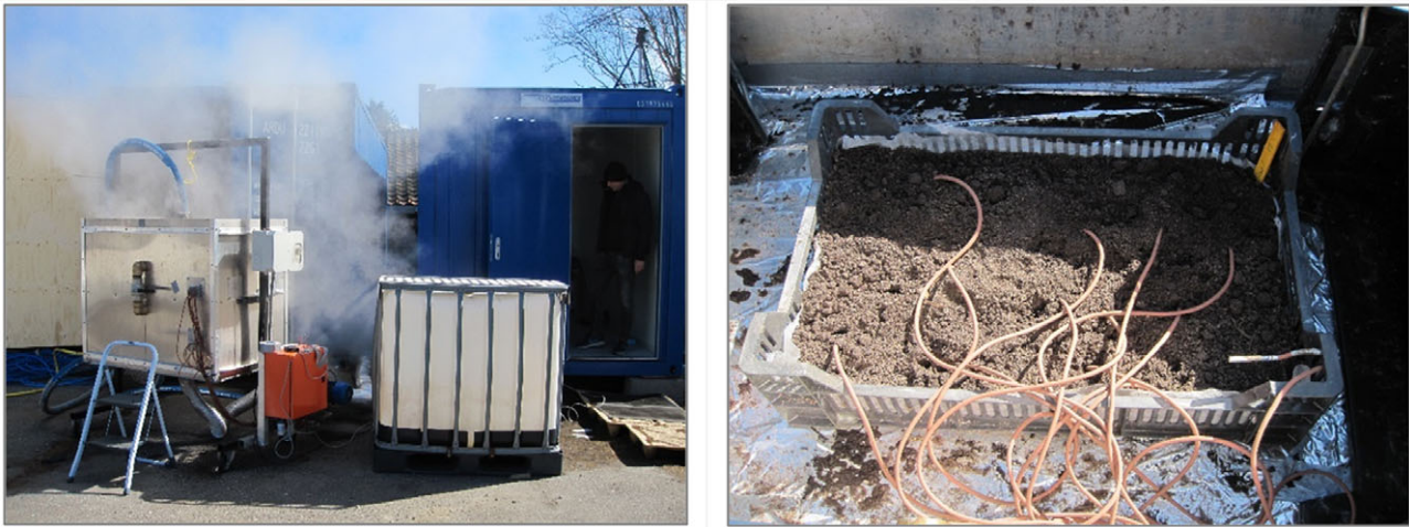
Figure 2. Steaming prototype device used in the experiments (left) and basket with soil, seed samples, and thermocouples placed inside the steaming container (right). Photograph by Vinh Hong Le.
