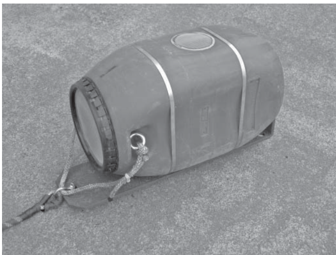
FIGURE 2. Photograph of the food-grade polyethylene drum used to cage individual rockfish showing the screens and bracket.
