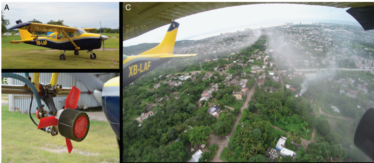
Fig. 2. (A) Aircraft employed in the trials with (B) the rotary atomizer mounted under wing and (C) aerial view during the application.
