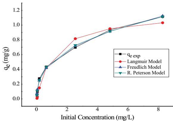
**Figure 9.** Isotherms of adsorption of phosphate onto pumice.
