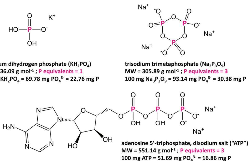
**Figure 3.** Chemical compounds used in this study to make in-house mixed-P standard solutions.  $\text{KH}_2\text{PO}_4$  dissociates readily to give phosphate anions that are detected in reactive P tests.  $\text{Na}_3\text{P}_3\text{O}_9$  and ATP each contribute 3 phosphate equivalents, but these molecules must undergo acid digestion to release phosphate anions.  $\text{Na}_3\text{P}_3\text{O}_9$  and ATP are thus detected in total P tests but are not detected in reactive P tests.
