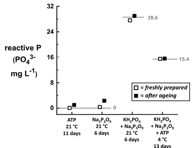
**Figure 6.** Comparison of reactive P results for freshly prepared samples (open symbols) and the same samples after ageing for several days (closed symbols) under laboratory conditions. Samples containing ATP and/or Na<sub>3</sub>P<sub>3</sub>O<sub>9</sub> show very small increases in reactive P when stored at 20 °C for 6 to 11 days. The 3-part standard solution showed no increase in reactive P after 13 days when stored at 4 °C.
