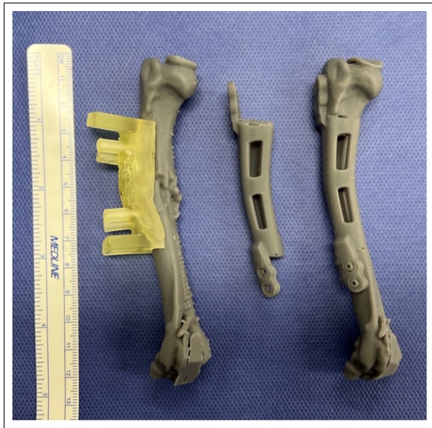
Figure 2 Three-dimensional printed bone models used to assist with surgical planning. Left: bone cutting guide affixed to the humerus with tumour. Centre: endoprosthesis. Right: three-dimensional printed endoprosthesis applied to the humerus after ostectomy of the humeral osteosarcoma
