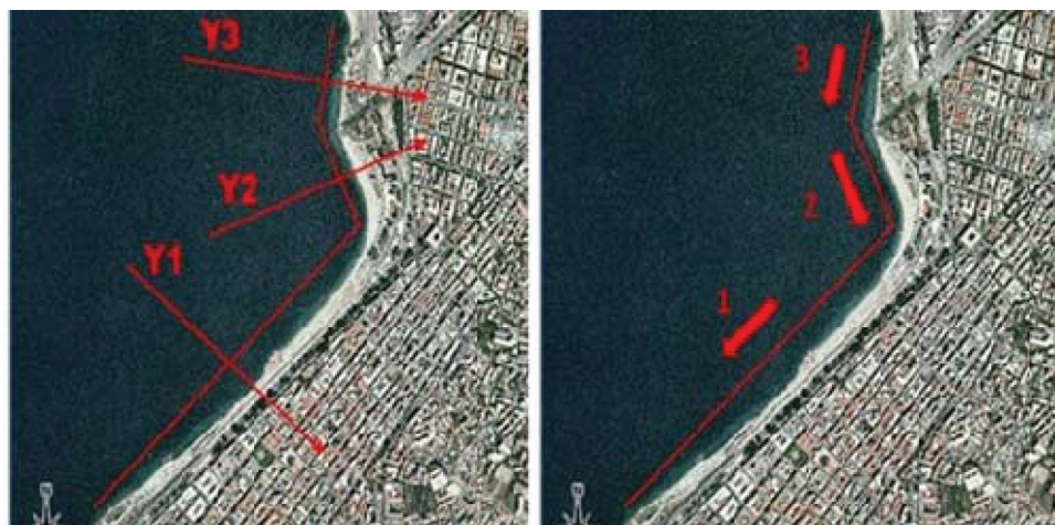
Figure 3. Sketch of the coast used in the simulation, and direction of the net longshore sediment transport.
