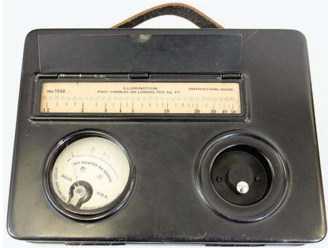
FIGURE 1. Picture of National Lamp Works foot-candle meter manufactured by General Electric in the 1920s and 1930s.
