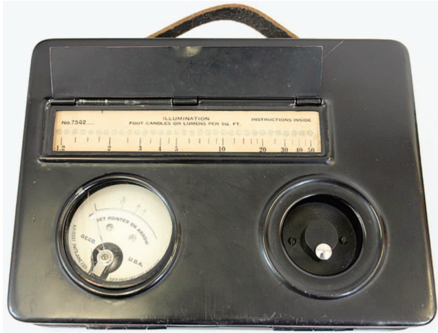
FIGURE 1. Picture of National Lamp Works foot-candle meter manufactured by General Electric in the 1920s and 1930s.
