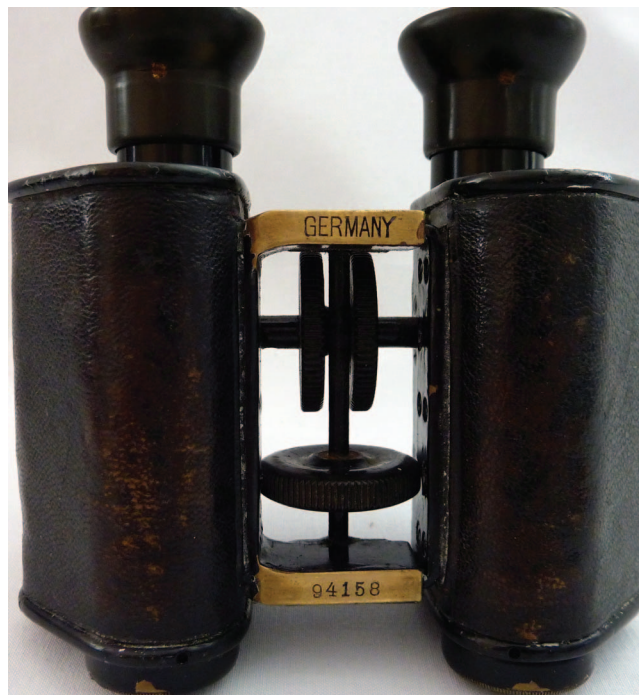
FIGURE 2. An example of the type of binocular that Huxley thought was too complicated to be used to watch birds. This is a Goerz 9×20 Trieder binocle no. 94158, manufactured in 1906. The lower wheel was for adjusting the distance between the eye cups and the upper two wheels were for focusing each eye piece independently. Photo copyrighted by Anna Vacani; used with her permission.
