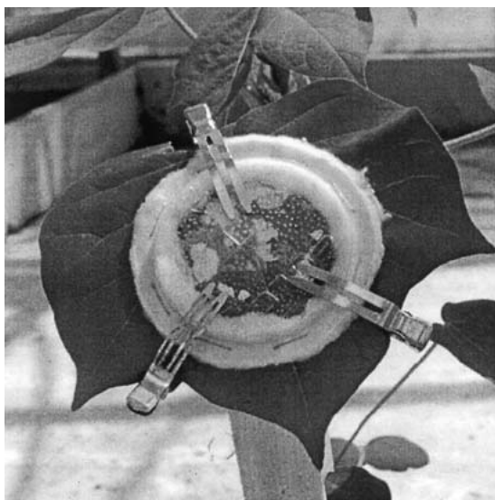
Fig. 1. Cage used to contain Spodoptera exigua larvae and resulting frass on corn or cotton leaves (cotton shown here) during herbivory trials (see text for description). Feeding damage can be observed through the perforated side of the cage. Cage was constructed of a pair of breathable plastic soft-drink lids, with the inside perimeter lined with cotton batting, held together by three curl clips.
